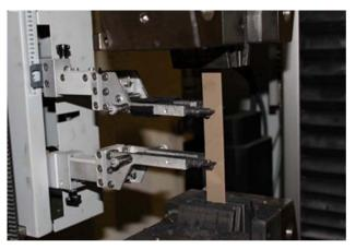
Figure 1. "Universal tensile strength measurement" apparatus with a cubic specimen.
