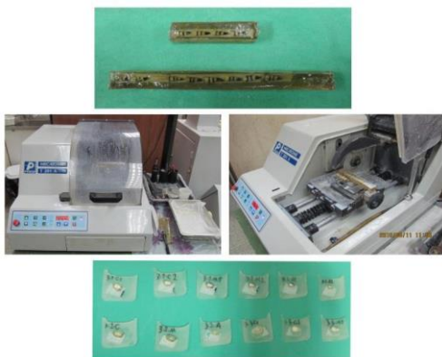
Figure 6. Cutting and mounting of specimens.
