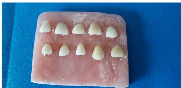
**Figure 2. Samples in heat-cured acrylic resin base.**
