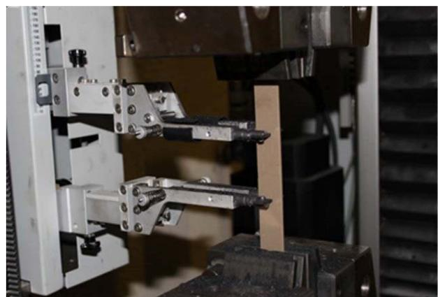
Figure 1. "Universal tensile strength measurement" apparatus with a cubic specimen.
