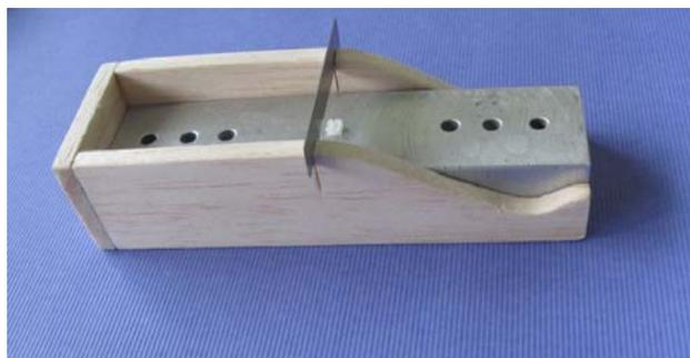
**Figure 1.** The method used to fix the bracket on the aluminum plate.
