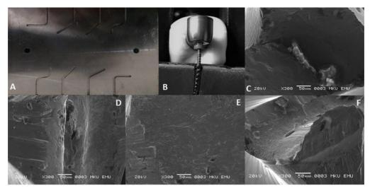
Figure 1. (A) Photograph of canal metal block. (B) Photograph of cyclic testing device used for the fatigue test. Representative SEM appearances of the (C) Race, (D) HyFlex CM, (E) FlexMaster and (F) Xp-endo Shaper files after cyclic fatigue testing (×300, original magnification).
