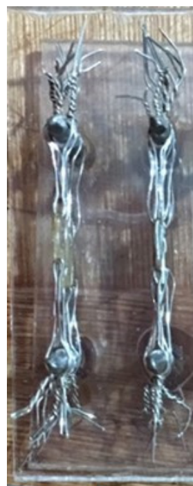
Figure 1. The two types of active tiebacks were stretched so that they exerted 250 g force initially at the 24 mm extension.
