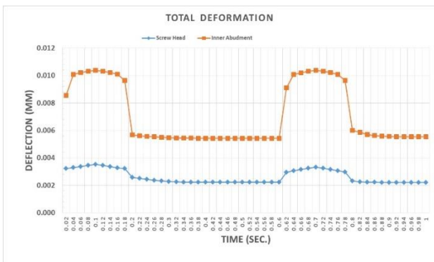
Figure 11. Comparison of minimum displacement of the screw head and the internal part of the octagon abutment at their interface during preloading and vertical loading.
