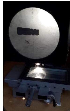
Figure 1. The profile projector.
