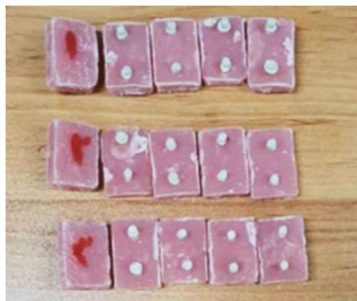
Figure 1. Samples mounted in Acropars 200 cold-cured acrylic resin, Iran
