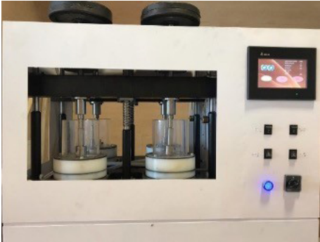
Figure 2. Nemo wear machine used to simulate mastication
