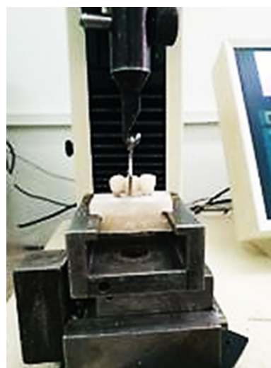
Figure 1. Pull-out test on a universal testing machine
