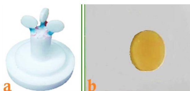
Figure 2. LD pressable ceramic discs fabrication: a) Spruing the milled wax pattern discs, and b) IPS e.max Press disc
