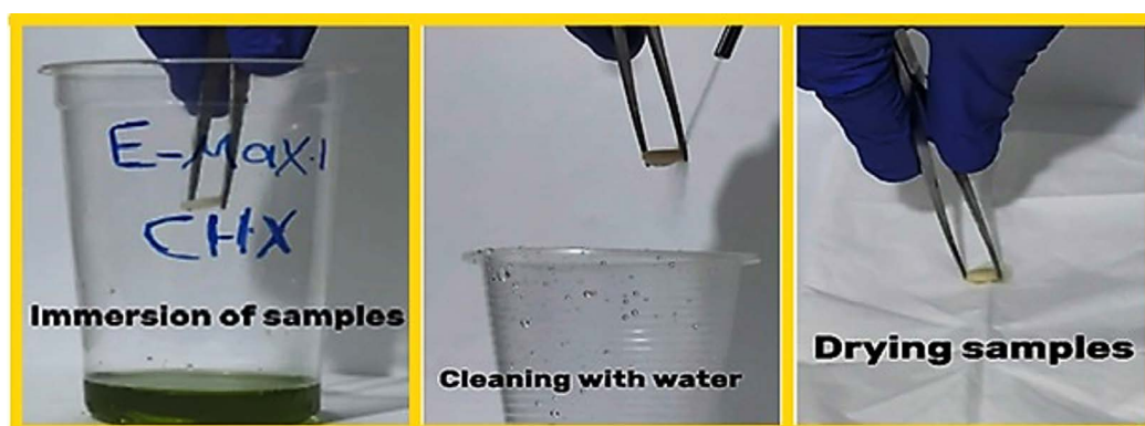
Figure 3. Sample cleaning and drying before testing
