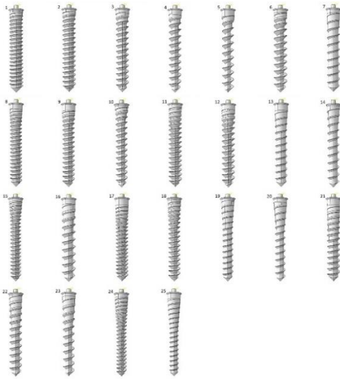
Figure 5. Twenty-five models of mini-implants for the Taguchi method, the second set of the models.
