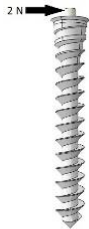
Figure 2. Application of a 2-N force at the head of the MI.
