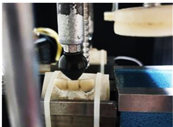
Figure 3. Forces on the bridge during the fatigue test
