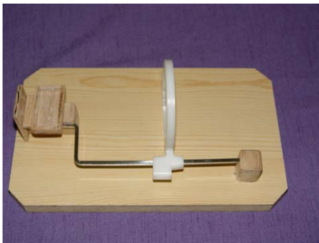
Figure 1. The optical bench which was constructed and used as a film holder.
