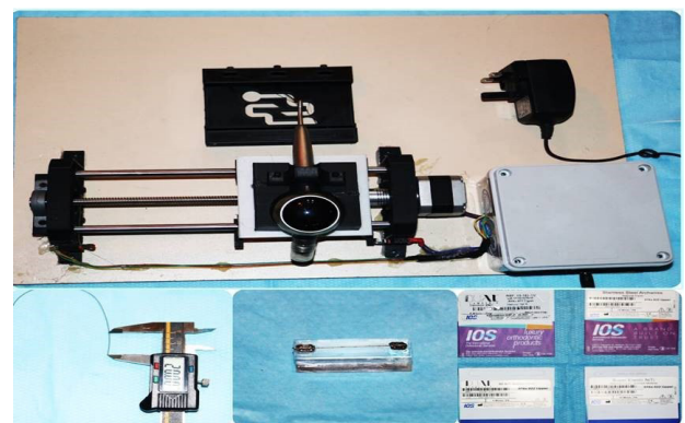
Figure 1. A customized holding device for air polishing, length of wire used, CNC block with wire attached to it, and archwires used
